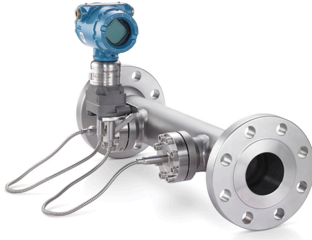
Figure 6. The Rosemount 9195 Wedge Flow Meter comes in standard, abrasive, and high and low temperature models for measuring flow in difficult slurry, viscous, hot, and coating/plugging processes.
