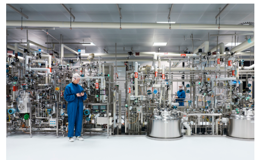
Image 1. Pharmaceutical skid with Emerson measurement instrumentation
